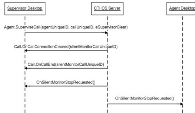
Figure 12: Message Flow When Ending a CCM-Based Silent Monitor Request
