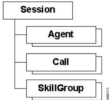
Figure 6: CIL Object Model Object Interfaces
